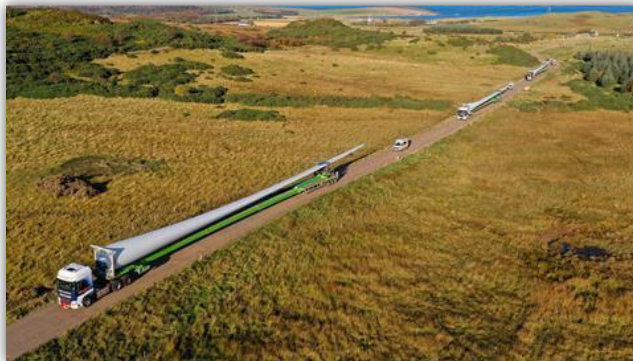
Turbine logistics [MotorTransport]
